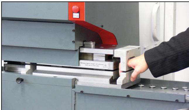
Fast blanking-tool change with side extension table for M-Cut 65
